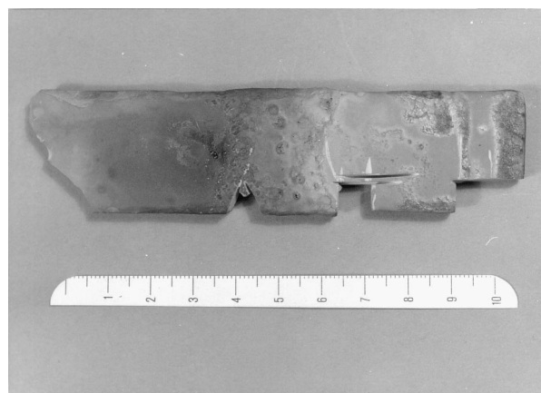
Fig. 3. Material A (dense zirconia) after corrosion test at 1550°C for 120 min, region I at positions 8.7–9.7, region II at positions 6.3–7.4 and region III at position 10.
